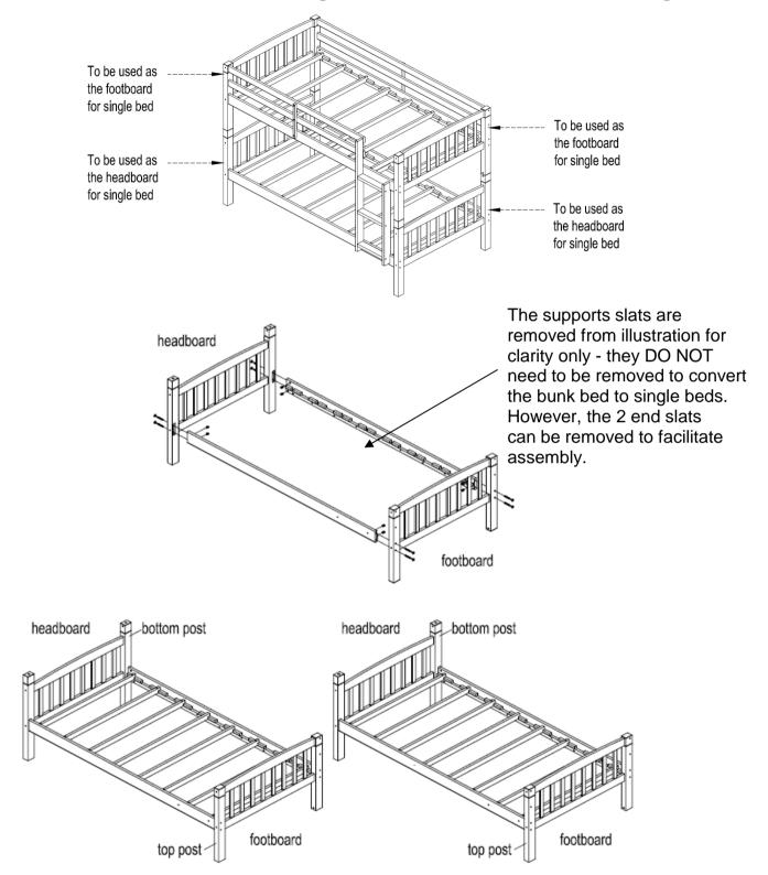
Remove the ladder and all the guardrails.
