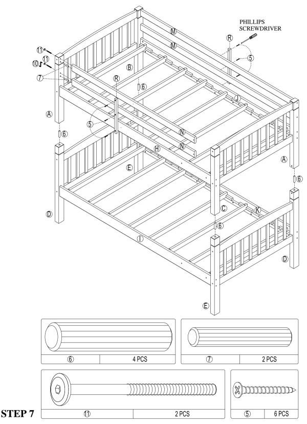
Place four wood dowels (6) into the holes in the bottom posts (D and E). With the help of another person, stack the top bunk onto the bottom bunk.
